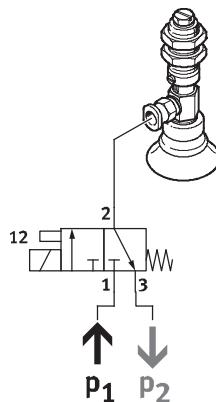
With the 3/2-way valve, normally closed, vacuum operation is established by connecting the vacuum (P2) to port 3 and connecting e.g. a silencer for venting (P1) to port 1. This changes the normal position from "closed" to "open".
